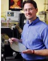
John Cressler holds a silicon-germanium integrated circuit wafer populated with nano-engineered SiGe circuits designed for a space environment. Behind him is a high-frequency test system used to measure the devices.
